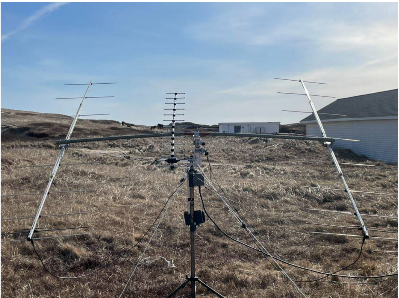
The EME aerial on Sable Island (FN93XW): Two 9 ele yagis for 2 m plus the 15 ele for 70 cm.
