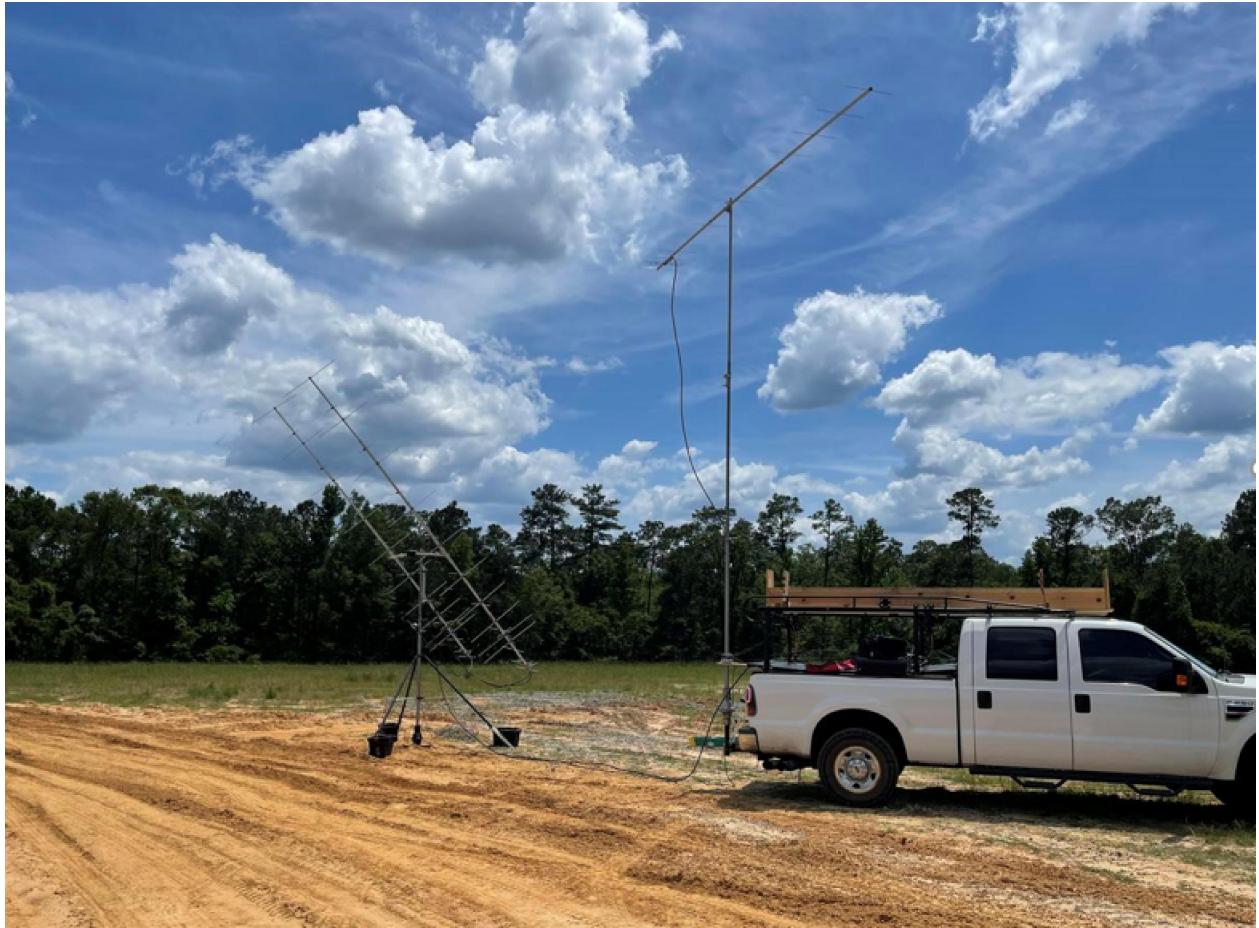
Peter's setup for 2 m EME and 1,25 m. Entire configuration can be broken down and packed within < 45 minutes.
