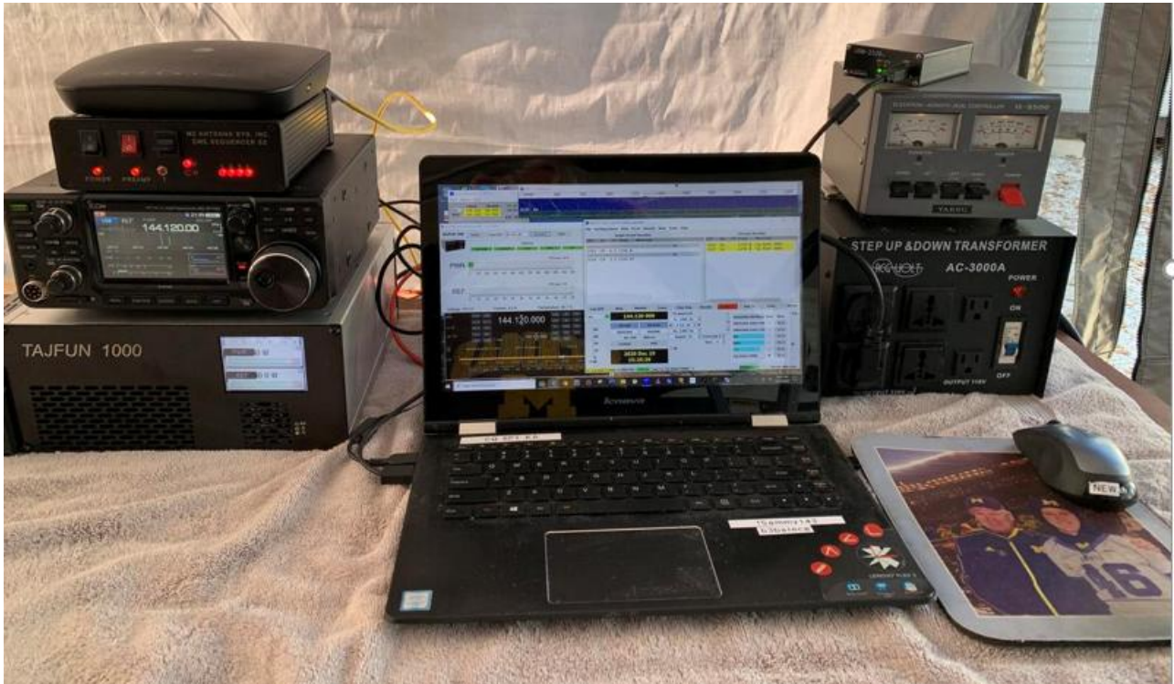
View on KA6U's updated station with the Tajfun 1000 SSPA running some 950 watts on JT65 with conditioning air blowing in the front. Everything fits on the driver's seat in the car.
