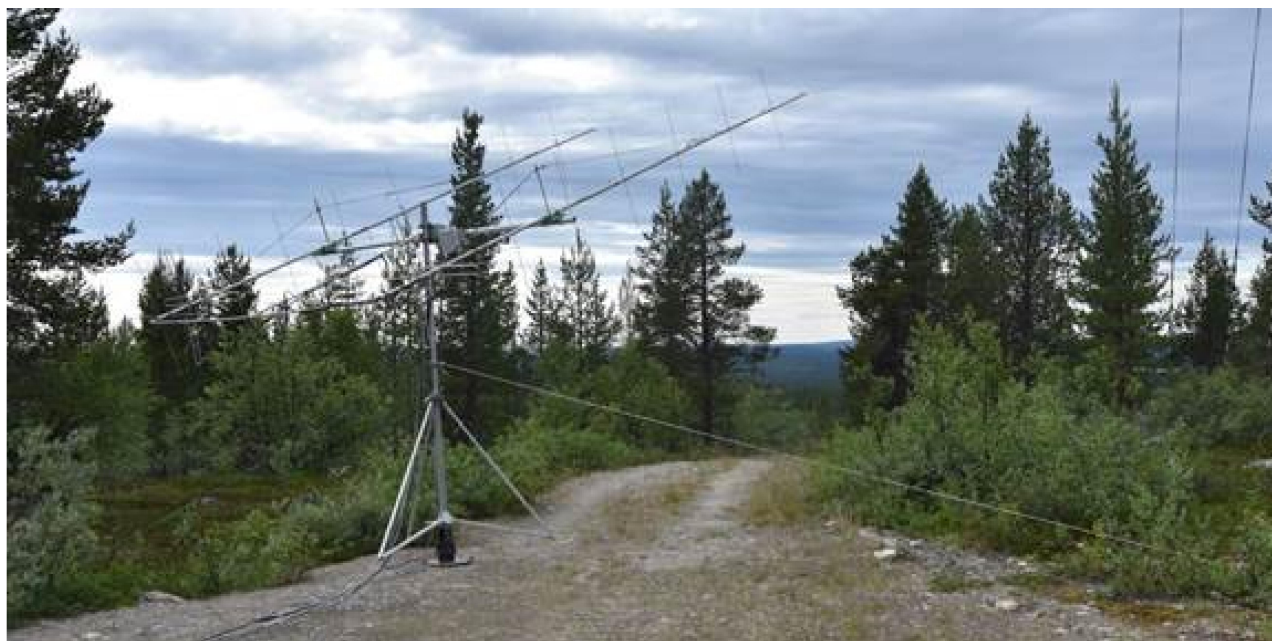
Jussis 2x11 hpol/2x10 vpol yagis in KP49EI: To the right you can see some commercial transmitting towers which made a little QRM when the moon was right in that direction but OH6ZZ still found a silent frequency to work.
