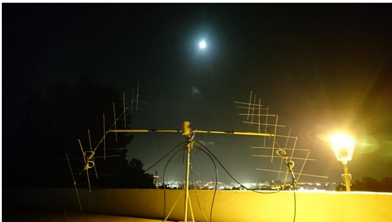
View to Ceuta from EF9LZ's antennas – two 8/8 ele xpols DK7ZB design
