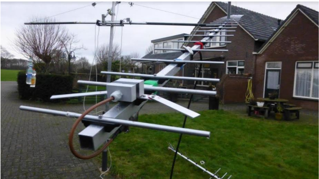
The newly built 70 cm antenna, being tested at Chris' place.
