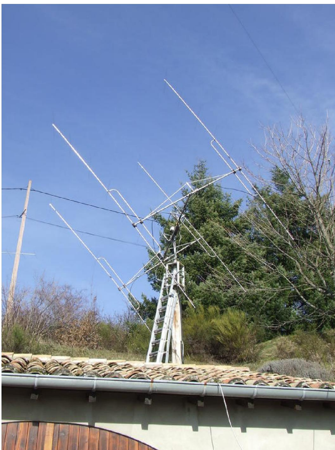
TM8DO/F8DO's 2 m antennas: 4x11 element Flexa modified (5.5 m long)
