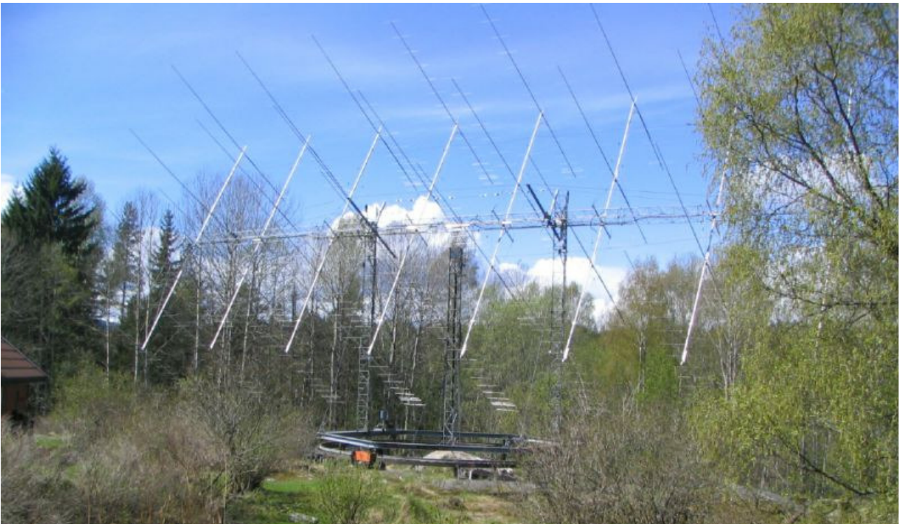
Facing an unsure future: Finn's fabulous 32 yagi array, one of the biggest in the world. (Photos LA3LF)
