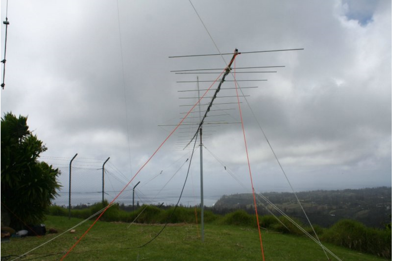
In its full shape: the VK9NA EME antenna pointing to the sea ( www.vk9na.com )
