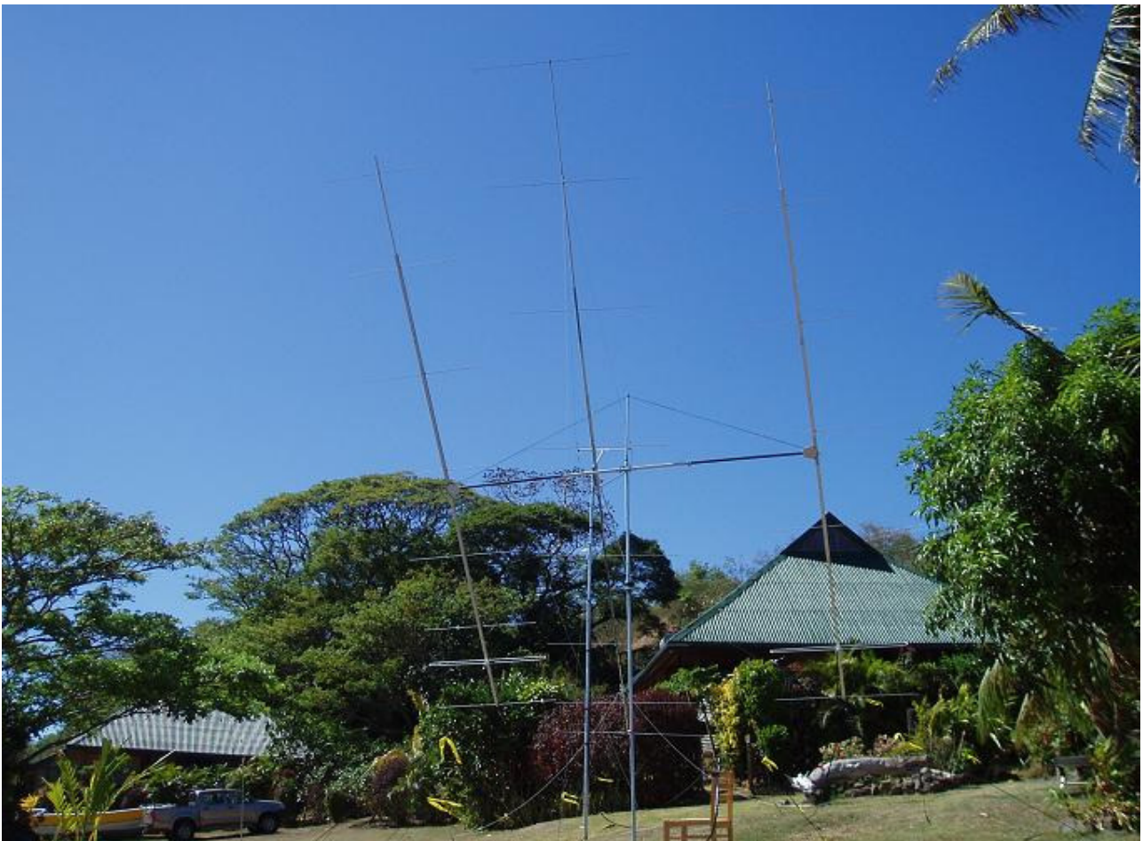
The 2 x 8 element yagis ZL1RS design and Lance's 6M8GJ yagi in the background. (ZL1RS)
